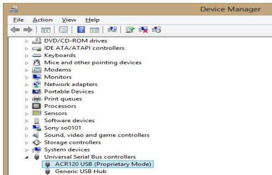
Gambar 10. Penginstalan driver ACR120U berhasil
