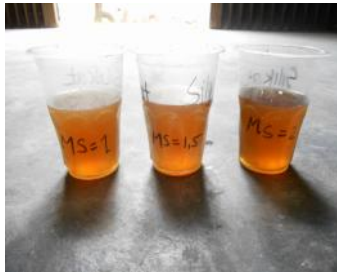
Gambar 2. Larutan Alkali Aktivator Sumber : Davidovits, 1994
