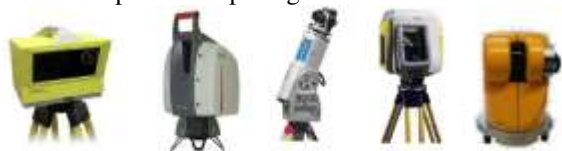
Gambar 2 Contoh alat Terrestrial Laser Scanner (Quintero dkk, 2008)
