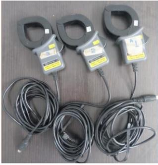
Gambar 2. Clamp Probe M-8125
