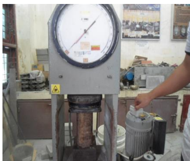
Gambar 4. Alat Compression Test Machine
