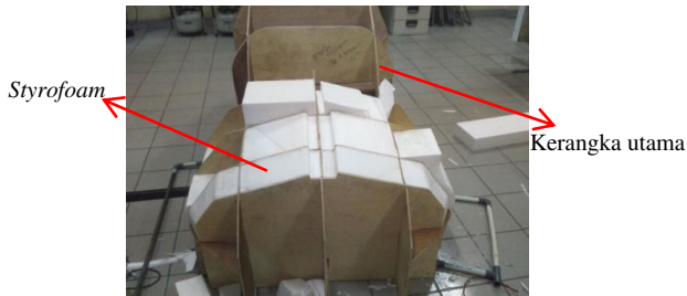
Gambar 9 Proses pengisian Styrofoam .
