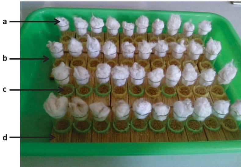
Keterangan (*Remarks*): a= kapas (*cotton*); b= semprong kaca (*glass pipe*); c= rayap (*dry wood termites*); d= contoh uji bambu (*bamboo specimen*)
