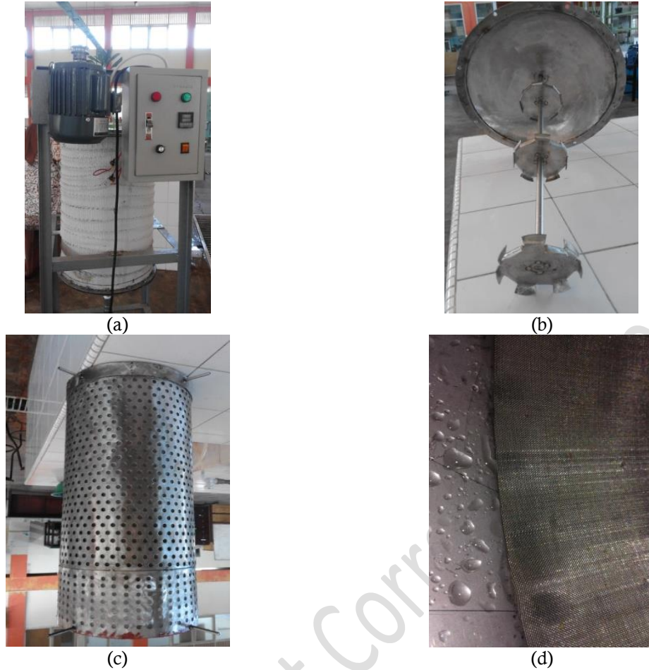
Figure 1. Extractor and its equipment (a) Extractor; (b) chopper and top; (c) outer filter; (d) inner filter
