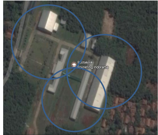
Gambar 8. Perancangan masing-masing radius ( r = 30m ) proteksi gedung kampus
