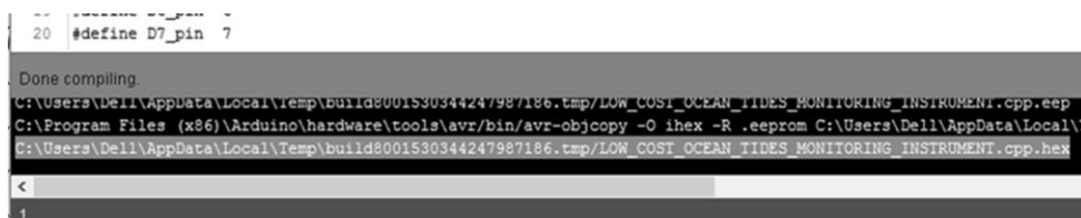
Fig 5. File path of hex file after compilation complete
