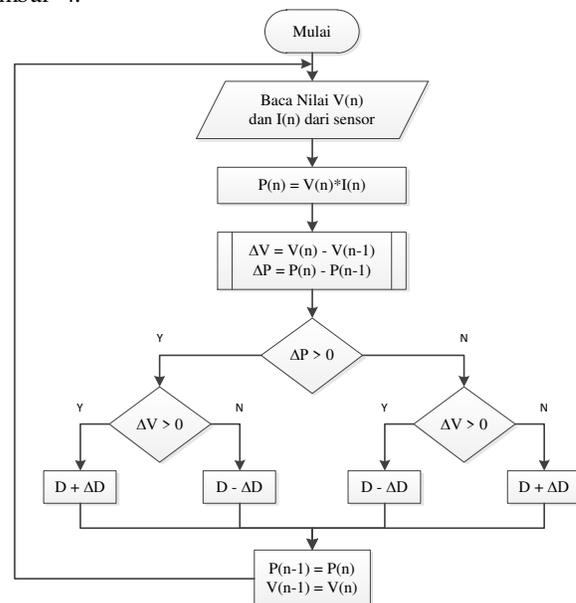
Gambar 4. Flowchart metode perturb and observe
