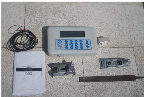
Gambar 7. Kesatuan Alat *Ultrasonic Flowmeter iSolv TUF 339*
