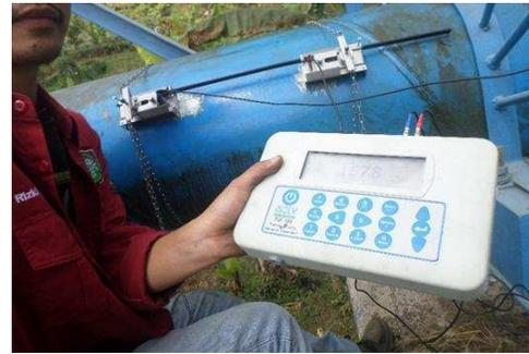
Gambar 8. Pengoperasian *Ultrasonic Flow Meter*
