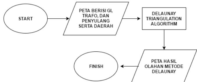
Gambar. 4. Diagram alur memodelkan Delaunay Triangulation Algorithm
