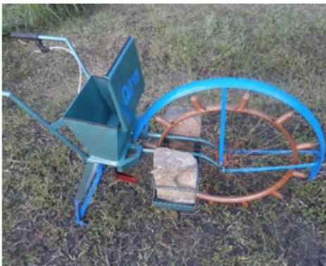
Gambar 3. Alat Q-Dros (*Quick Drop Seeder*)
