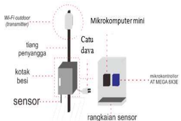
Gambar 3. Desain wireless sensor network
