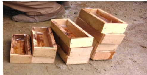
Gambar 2 Bekisting sampel uji korosi
