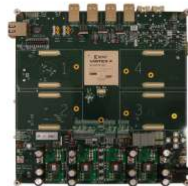
Gambar 2.2 Perangkat Wireless Open-Access Research Platform
