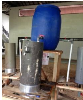
Gambar 1. Prototype septic tank
