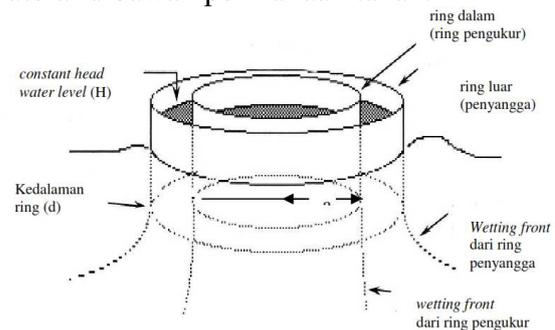
Gambar 3 *Double Ring Infiltrometer*
