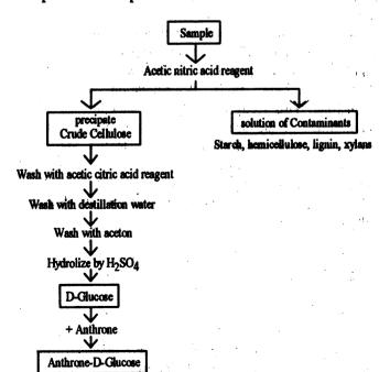
Concentration is detected using a Spectrophotometer at 620µ
