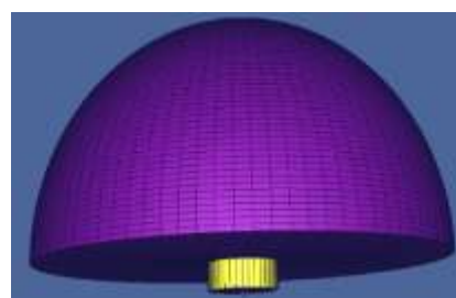
Fig. 8. MCNP Visual representation of NaI(Tl) detector with radiation source R= 3 m.
