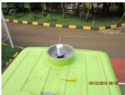
(b) NaI(Tl) detector at the vehicle roof
