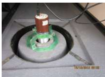
(a) NaI(Tl) detector at the vehicle floor
