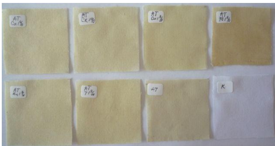
Figure 4. Cotton cloths dyed with A. terreus dye using different mordants; Ca = \text{CaCO}_3 , Cr = \text{K}_2\text{Cr}_2\text{O}_7 , Cu = \text{CuSO}_4 \cdot 5\text{H}_2\text{O} , Fe = \text{FeSO}_4 \cdot 7\text{H}_2\text{O} , Mn = \text{MnSO}_4 \cdot \text{H}_2\text{O} , T = alum, K = control.
