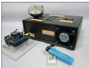
Fig. 14. Overall model configuration of the wireless gas leakage monitoring system with the gas detector.
