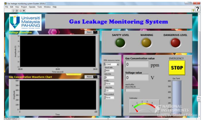
Fig. 3. The GUI of monitoring the gas leakage.
