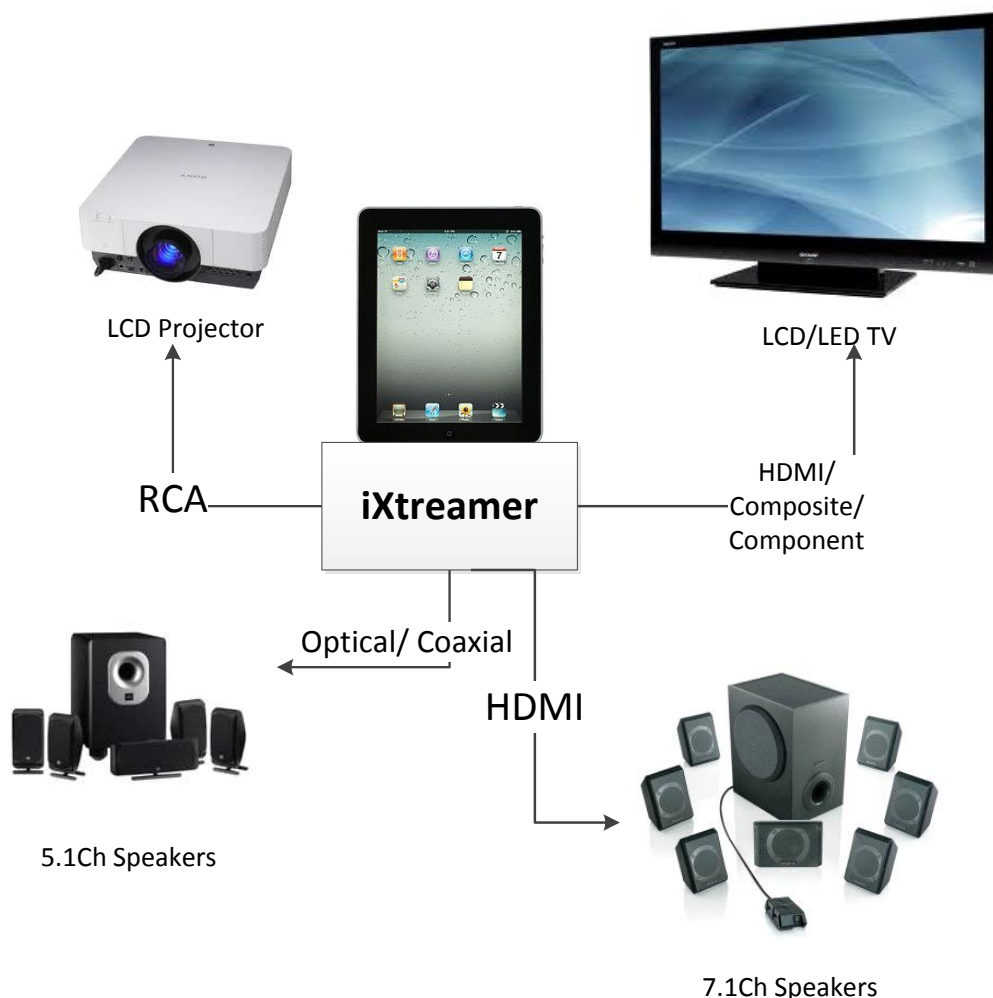
Figure 2. shows diagram of the combination of iPad and iXtremer.
