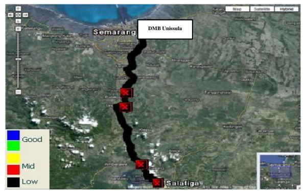
Fig. 5. The Result of the Main road drive test in the Southern Area
