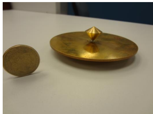
Figure 2 UWB monocone antenna with ground plane of 100 mm
