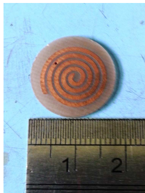
Fig. 2. Picture of realized compact circularly spiral planar inverted-F antenna
