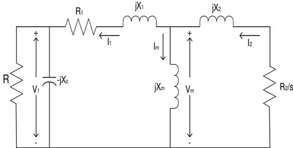
Fig. 4. Equivalent circuit at fundamental frequency of a single-phase induction generator under loaded condition in stand-alone operation [13]
