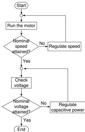
Fig. 8. Algorithm to regulate generator speed and voltage.
