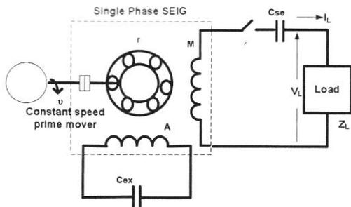
Fig. 1. Self-excited single-phase induction generator with capacitors connected to both the main- and auxiliary-windings [9].
