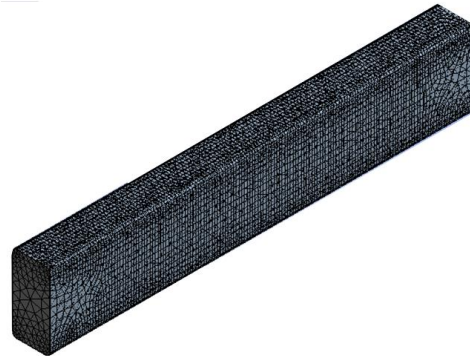
Figure 2. Meshing for Composite Sandwich Specimen
