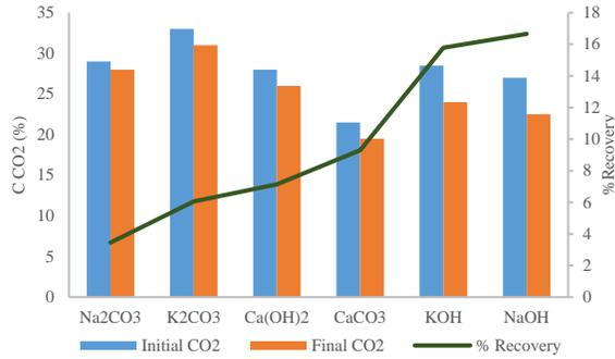
Figure 1. % Recovery of CO<sub>2</sub> from various absorbents.
