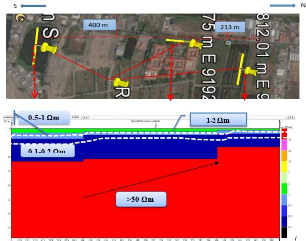
Figure 7. Subsurface Model of VES
