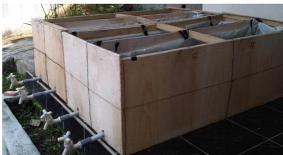
**Gambar 1. Reaktor SSF-Wetland**
