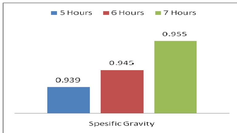
Figure 3. Specific gravity of Patchouli oil influenced by distillation length.
