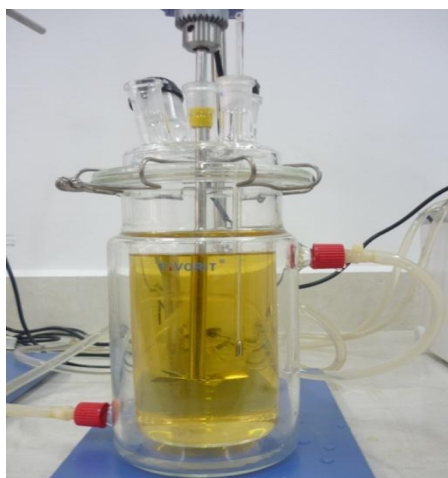
Figure 2: Experimental setup of esterification and transesterification process.
