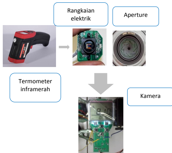
Gambar 8. Skema Perancangan Prototype Optical Thermometer
