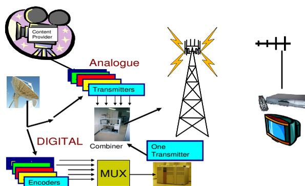
Figure 1 The scheme of DVB-T system (Roddy, 2006)
