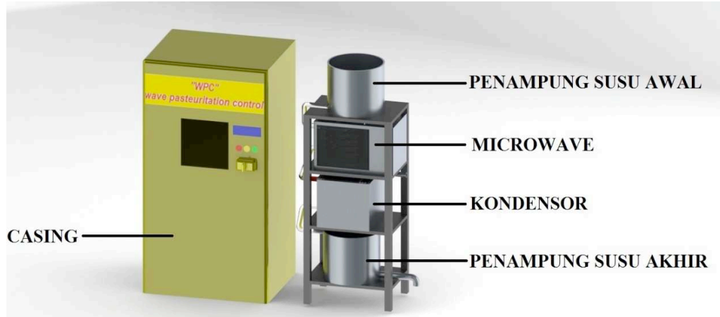
Gambar 2. Desain WPC ( wave pasterutiation control )
