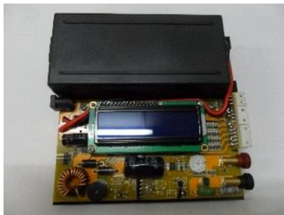
Gambar 9. Rangkaian BCR (Battery Control Regulator)
