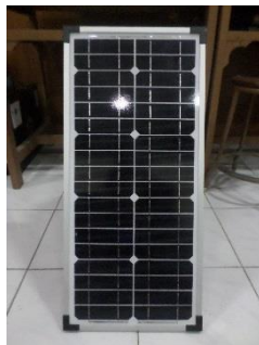
Gambar 10. Panel Surya 20 Watt
