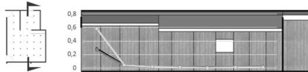
North-South Section of Daylight Factors on Bilik 1 room
