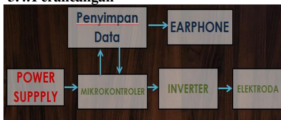
Gambar 2: Diagram Blok Sistem ALTERSIMEDIS
