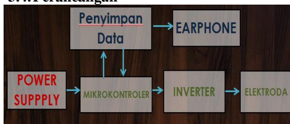
Gambar 2: Diagram Blok Sistem ALTERSIMEDIS
