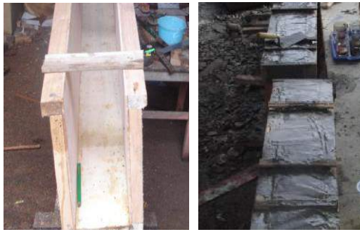
Fig. 5: Test preparation materials and casting beams
