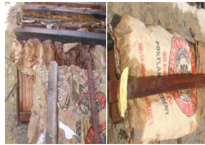
Fig. 7: Curing specimen beams
