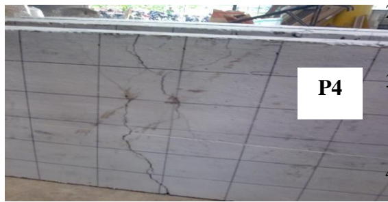
Figure 9: crack pattern test specimens
