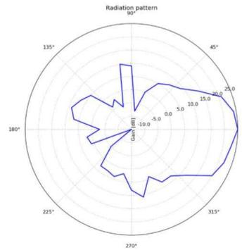
Gambar 2. Pola Radiasi Antenna Wifi
