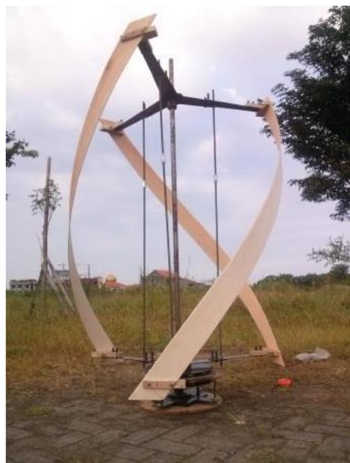
Gambar 7. kiri : Hasil akhir turbin Heliks. kanan : Proses *outdoor testing* turbin Heliks
