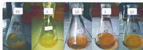
Fig. 3. Hydrocracking Product of Catalyst Weight Variation
