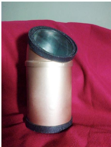
**Gambar 23.** *Prototype Light Tube Horizontal – Pendek (1)*
