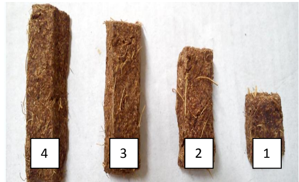
Gambar 1. Batangan Filter Diesel Particulate Filter (DPF)
