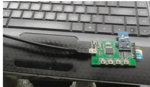
Gambar 3.7. Instalasi IQRF coordinator
