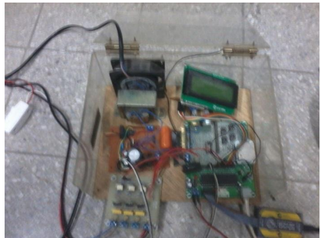
Gambar 4.5 Single Phase AC Induction Motor Controller
