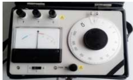
Gambar 6. Earth Resistance Tester
